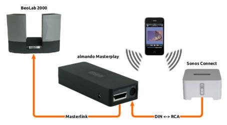
As soon as you start the playback on the Sonos Connect with your Sonos Control App, the almando Masterplay automatically activates BeoLab 2000. Naturally, playback is absolutely synchronous with other Sonos speakers in your Sonos Multiroom system without any time delay.
