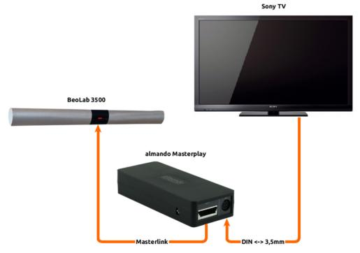
As soon as you switch on the TV with the TV remote control, the almando Masterplay automatically turns on the BeoLab 3500. You do not need a B&O remote control for this.
