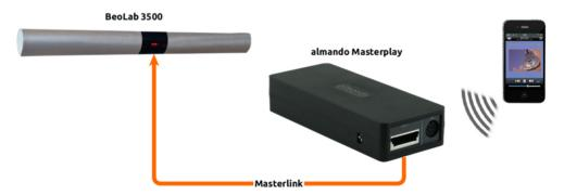
Of course you also can send the music wirelessly from your smartphone or tablet to the almando Masterplay via Bluetooth. The connected Masterlink speaker ist turned on automatically. You don't have to press any key on the speaker or on a B&O remote control - simply start any app like Spotify, Youtube, TuneIn Radio, etc. and off you go!
