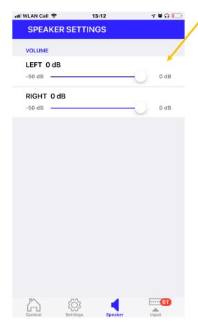
With these sliders you can adjust the individual volume for both speakers (LEFT and RIGHT). And these settings can be made separately for each input (BLUETOOTH, SPDIF, INPUT 1 and INPUT 2).
